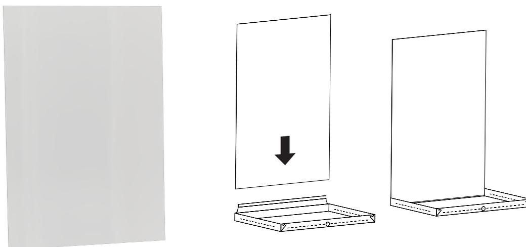
The wall panel is a sealing layer against walls that is customised to divert water leakage down to our leak protection such as Tollco Appliance Mat Pro and Standard, Tollco Wet Zone Floor Protection Dishwasher/Washing Machine, Floor Protection Base Cabinet or Tollco Base Cabinet Insert.
