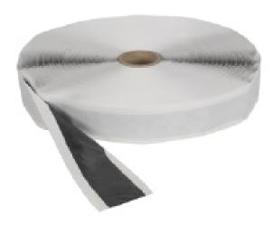
The black sealing tape is double-sided and made of polyisobutylene. Used to seal joints between two different materials, such as the cabinet bottom and a plastic floor protector.
