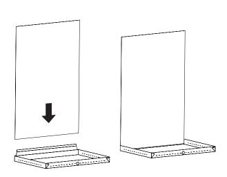
The wall panel is a sealing layer against walls that is customised to divert water leakage down to our leak protection such as Tollco Appliance Mat Pro and Standard, Tollco Wet Zone Floor Protection Dishwasher/Washing Machine, Floor Protection Base Cabinet or Tollco Base Cabinet Insert.
