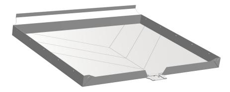
Floor Protection Dishwasher and Washing Machine is a closed tray that is placed under dishwashers/washing machines and sink cabinets. Collects water leaks from hidden areas and protects the floor from water damage. Can activate water circuit breaker if installed. Comes with outlet that can divert and make water leakage visible. To install the outlet, cut the front edge and attach the outlet. Available in several sizes and can be installed when renovating or building a new kitchen.
