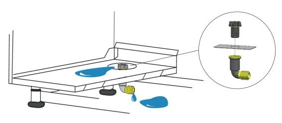
Flood Protection Mini-Drain with recess is a wastewater pipe mounted on the bottom panel of a base cabinet that creates a natural slope that diverts water away from hidden surfaces to a water-safe space. Install the mini-drain in the kitchen cabinet under a water heater, expansion tank etc. where water can leak.
